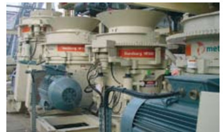
Stationary : One HP500, one HP300, two HP200 crushing "Amphibolite".
