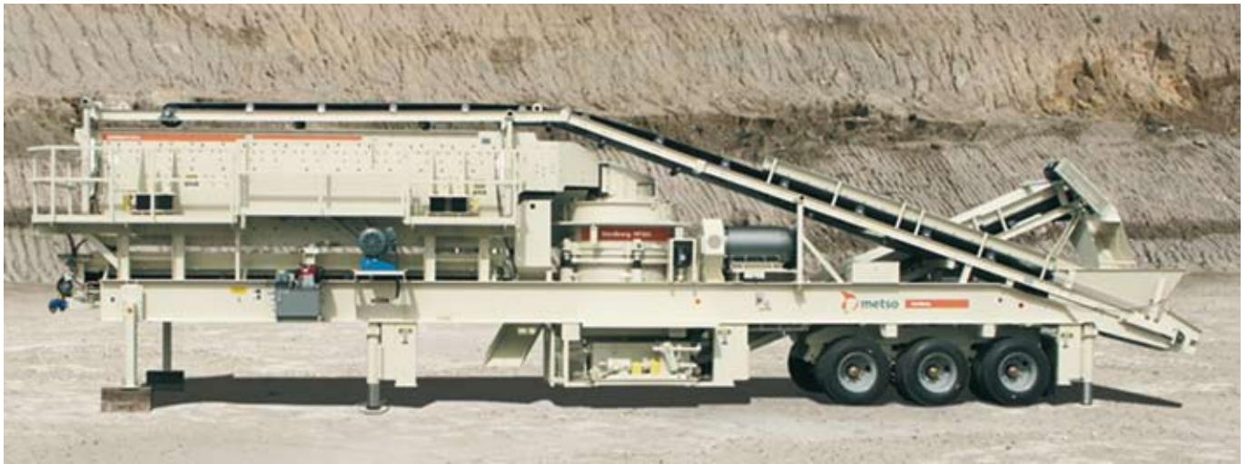
Mobile : The Nordberg NW300HP is a highly mobile, closed-circuit crushing and screening plant. Ideal for contractors, it can transform your feed stock into three finished fractions.
