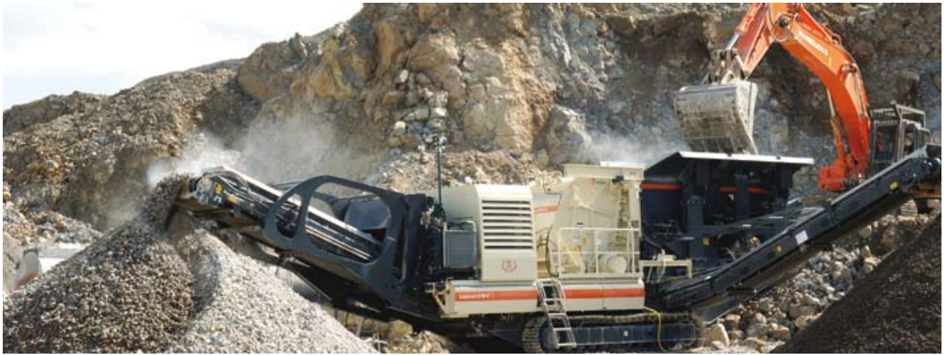
Mobile : The Nordberg Lokotrack LT1415 is built around the powerful NP1415M impact crusher.
